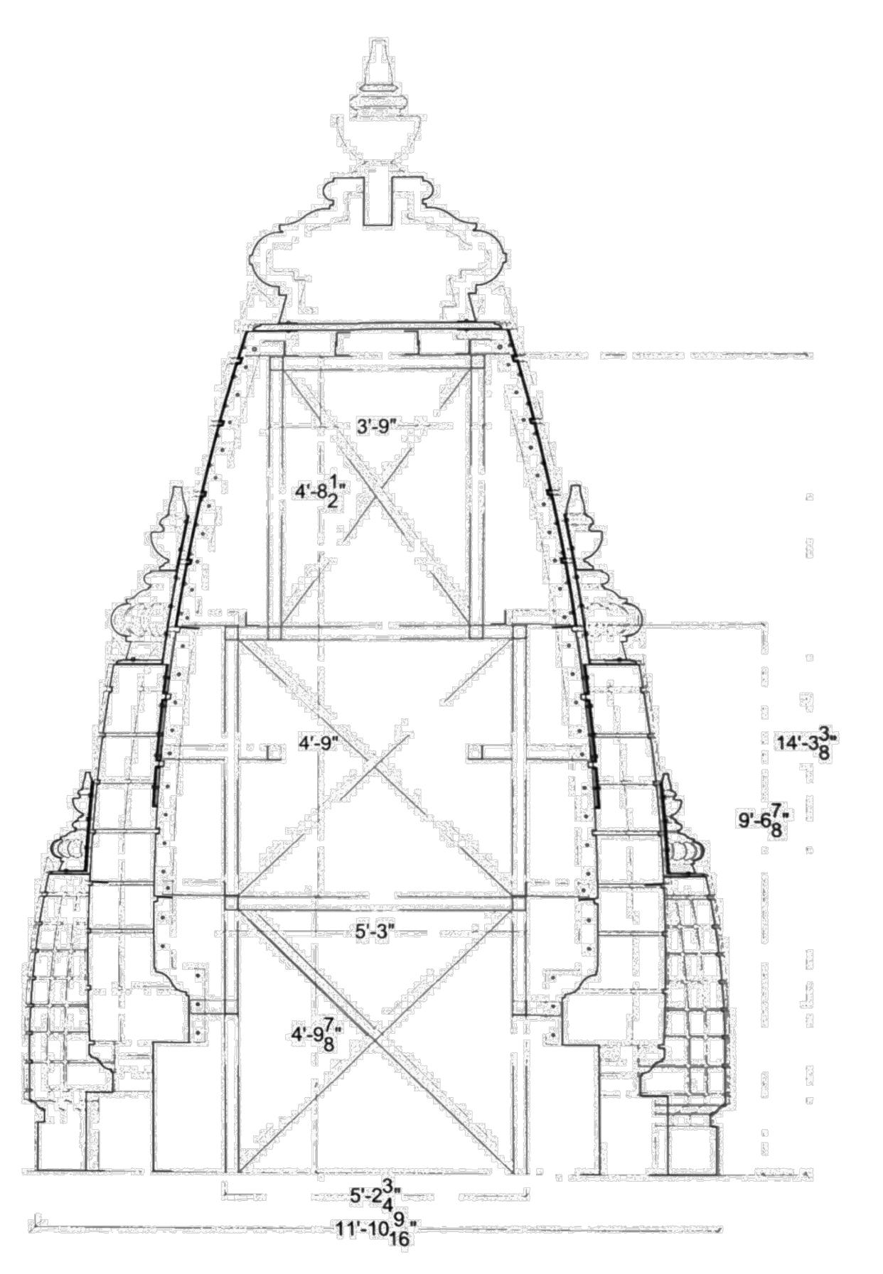
FRP SHIKHAR SECTIONAL ELEVATION WITH STEEL STRUCTURE Scale 3/4-11-07
