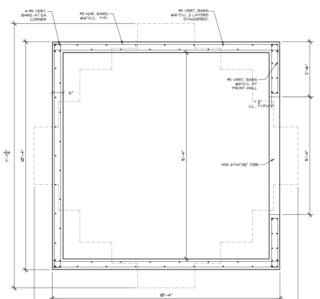
TOP OF CONCRETE WALL STRUCTURAL PLAN SCALE: N.T.S.
